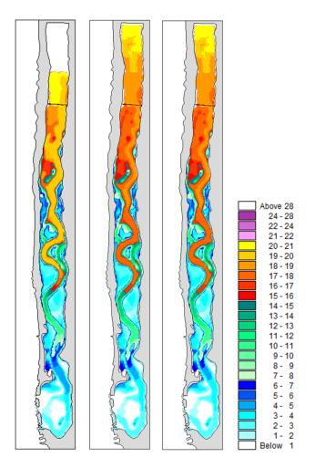
Local water renewal times in days for actual conditions (left), proposed removal of upstream dike (center) and proposed dredging of flood delta circulation channels (right) © DHI / Hydrosoft S.A. The models were calibrated against two-month long series of currents, water levels, salinity and temperature. These were measured at four different locations inside the lagoon. Also, waves at the entrance were calibrated against wave measurements of the same duration.
