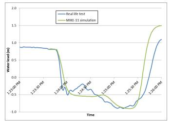
Comparison of measured water levels vs. MIKE 11 calculated water levels for a load rejection test. © Hydro-Québec
