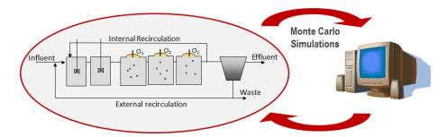
The Metcalf & Eddy guideline is used to size a predenitrification plant for nitrogen removal. An uncertainty analysis was performed on the design space by randomly sampling influent fractions, effluent requirements, and safety factors.
